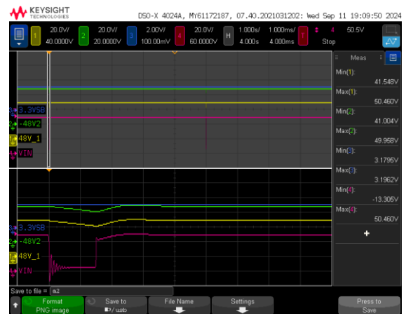
Fig. 5. Output Voltage Waveforms During UV Part of PDOT
