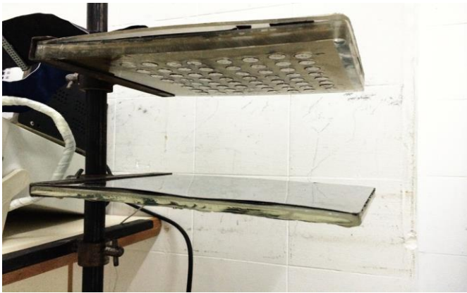
Fig. 1. Plexiglas plate containing embedded 64 electrodes for breast tissue electrical bioimpedance measurements
