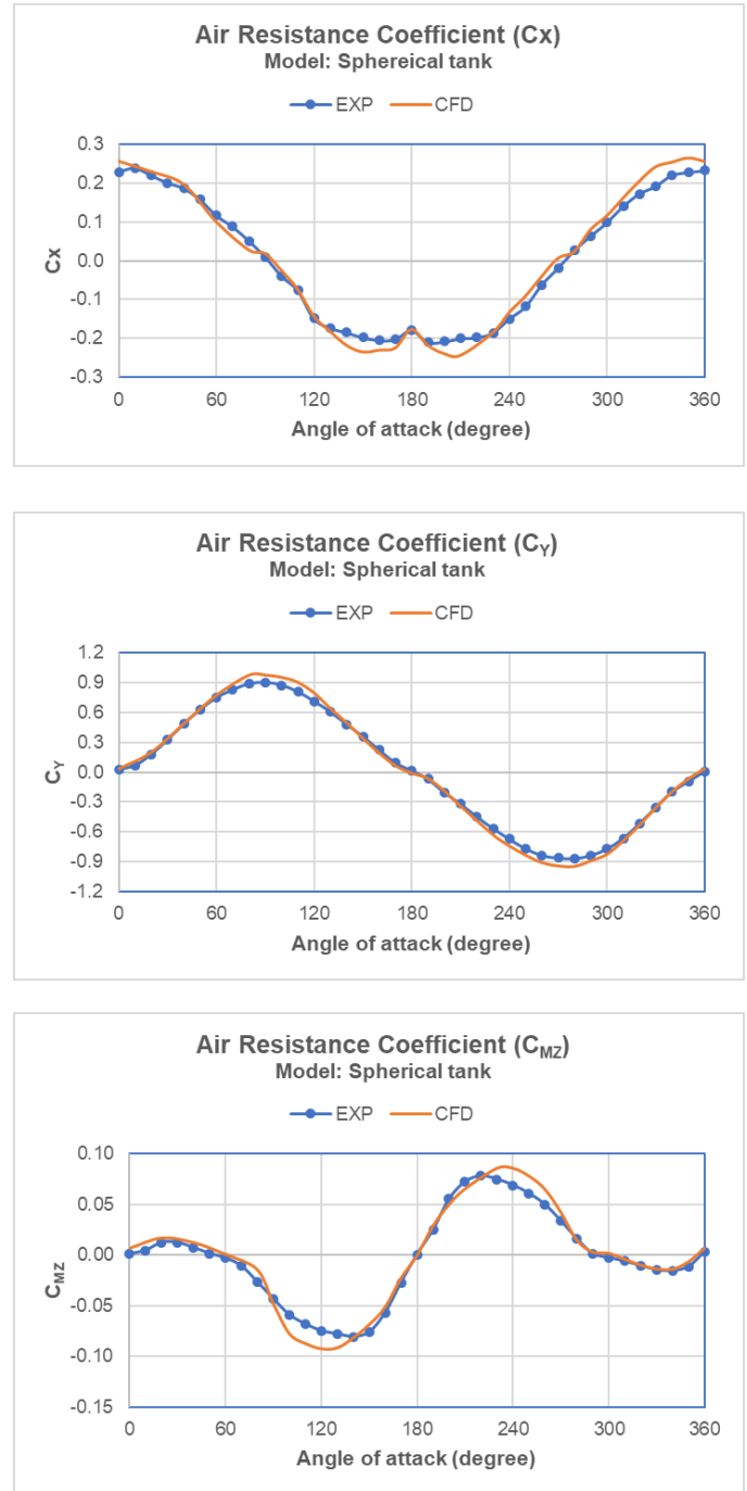
Fig. 8. Air resistance coefficient – spherical tank
