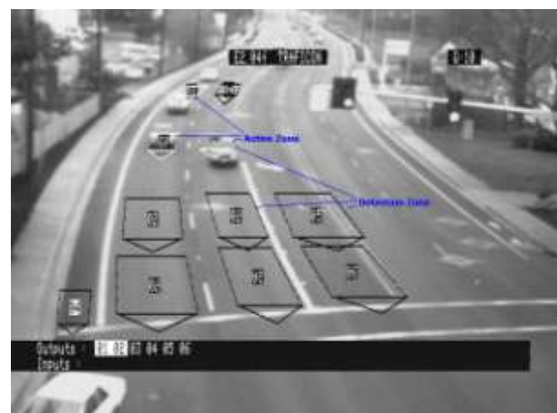
Figure 5. Video cameras at signalized intersections
