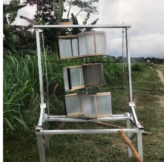
Fig. 14. Multi-level Savonius Wind Turbine with Independent Rotational Axis
