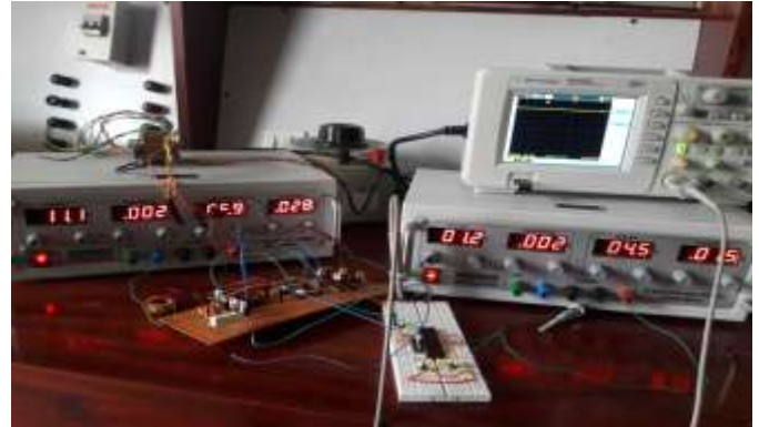
Fig. 25. Experimental setup for new transformerless buck-boost converter
