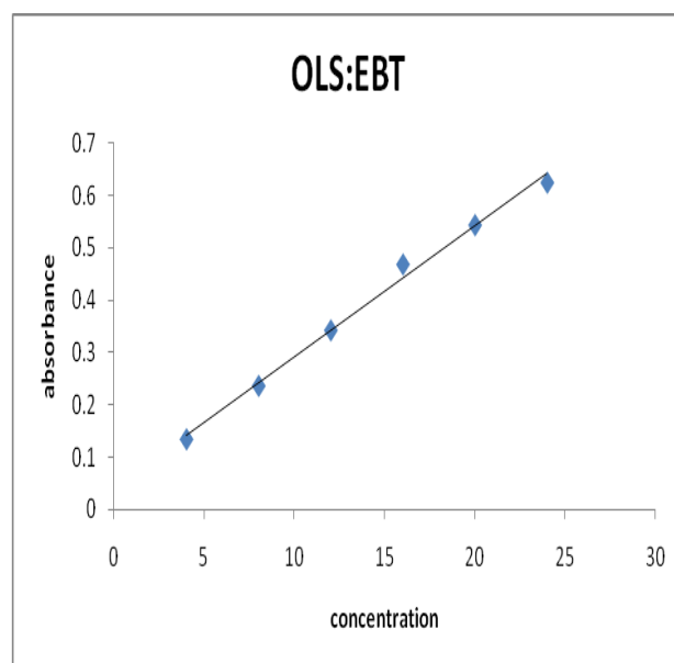
Fig 3a: Calibration curve of olmesartan with eriochrome Black-T.
