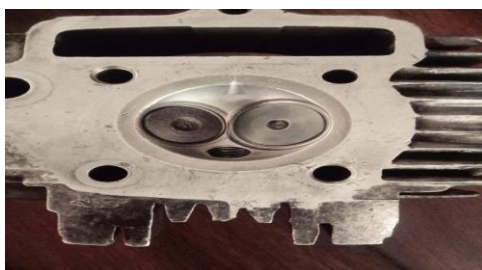
Figure 9 Cylinder Head Machined with Grooves
