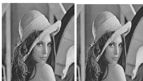
Fig. 3 Stego-images obtained by (a) LSB-substituted method; (b) proposed method, with secret-image is 4-bit inserted.
