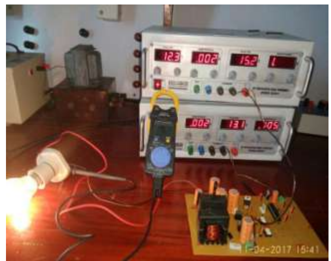
Fig 15. Experimental result showing MPPT operation
