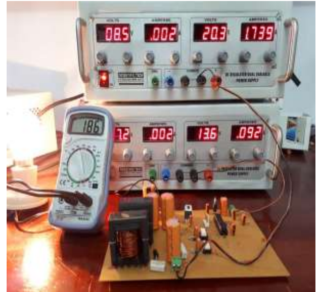
Fig 15. Experimental result showing voltage gain
