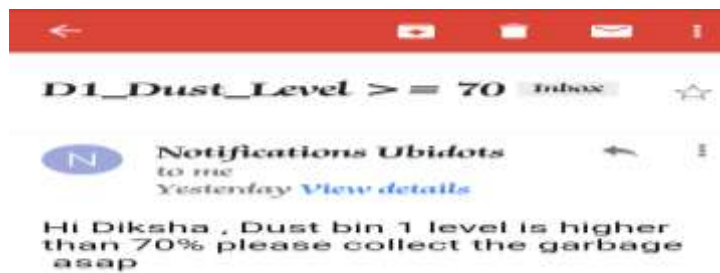
Figure 4.11: The alert E-mail Recived for dustbin 1 When the bins D1 is full, a notification or a E-mail is sent using cloud to the staff in-charge.
