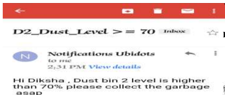
Figure 4.12: The alert E-mail Recived for dustbin 2 When the bins D2 is full, a notification or a E-mail is sent using cloud to the staff in-charge.
