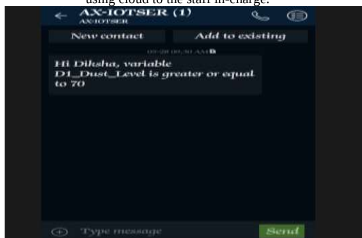
Figure 4.13 The SMS received in Message Box When the bins are full, a notification or a message is sent using cloud to the staff in-charge.
