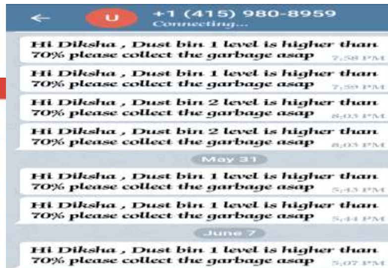
Figure 4.14: The Message received in Telegram apps When the bin D1 or D2 are full, a telegram is sent using cloud to the authority.
