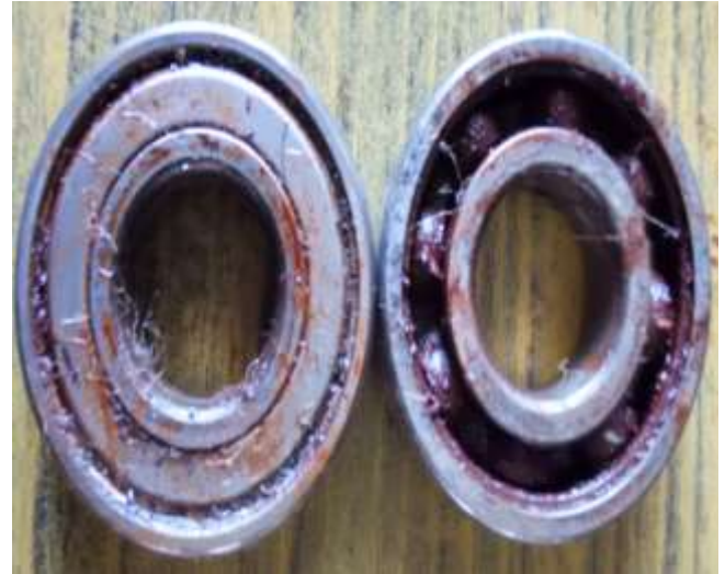
Fig 5.1 Healthy and faulty bearing
