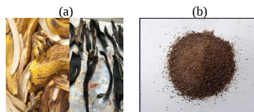
Fig. 1: Images of the: (a) fresh and sun-dried banana peels (b) powdered banana peels
