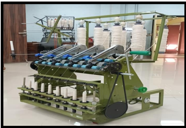
Figure 1: New Modified charkha
