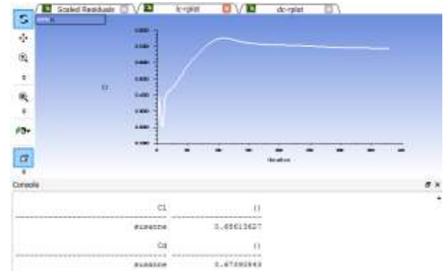
Fig.6. Coefficient of lift of Susanne at 40° AOA
