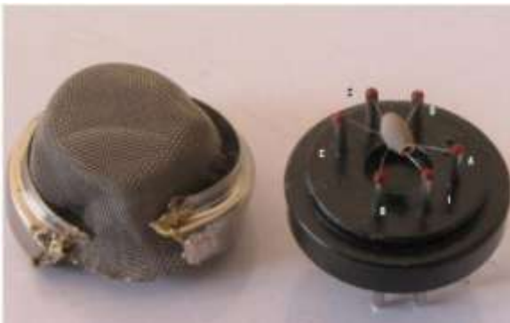
Image Showing Hexapod Structure inside a Gas Sensor
