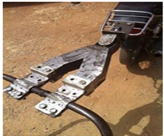
Fig. 7. Hitch Connecting Both Trailer and Motorcycle During Testing
