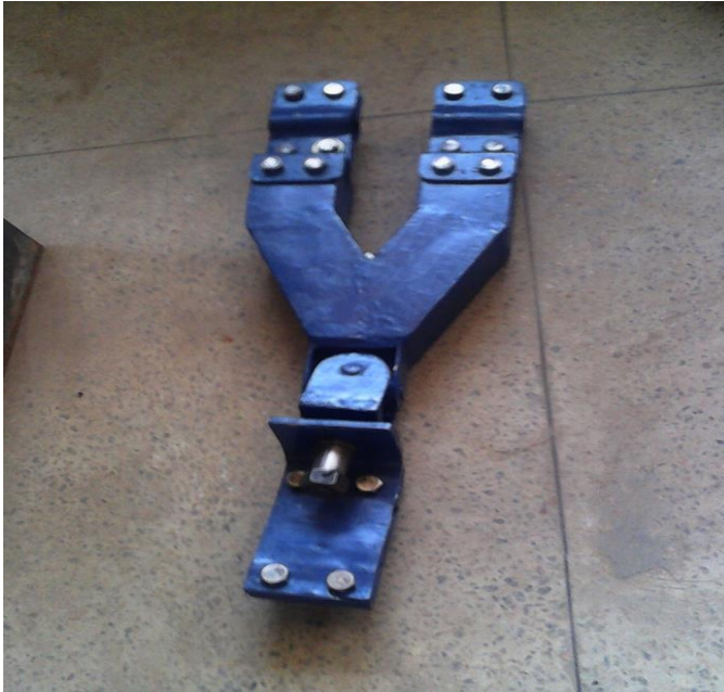
Fig. 8 Fully developed motorcycle trailer hitch
