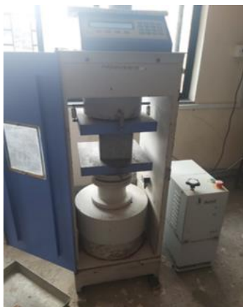
Fig -1 : Testing of Concrete cubes
