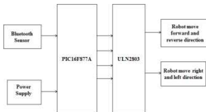
Fig. 2 Block diagram of Robot with Bluetooth sensor [4]
