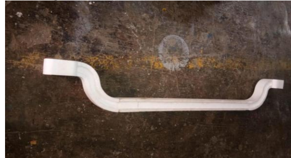
Fig19- Thermocol Pattern CASTING PROCESS
