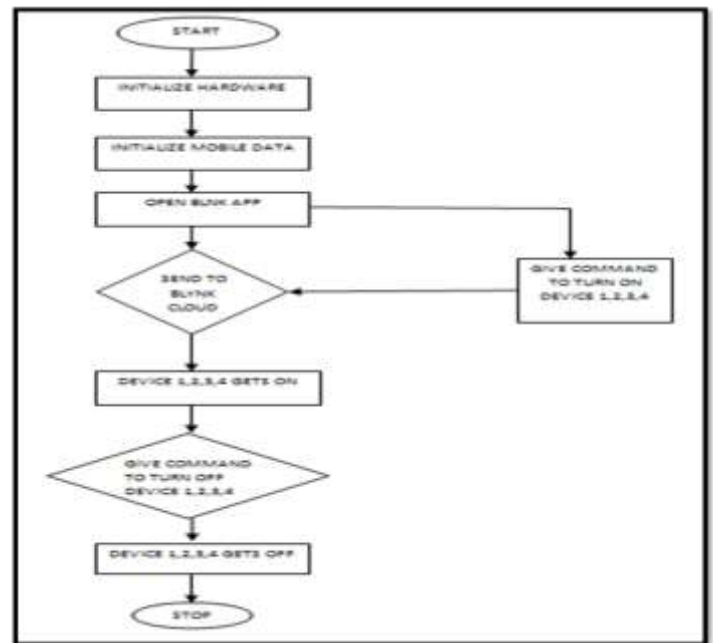
Figure 5: Home automation using BLYNK app
