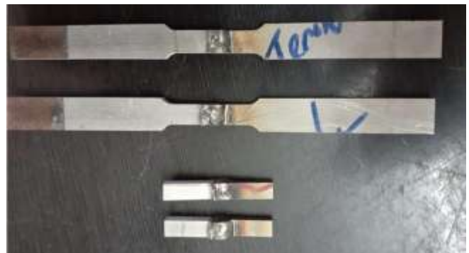
Fig. 3. Tensile and hardness testing samples
