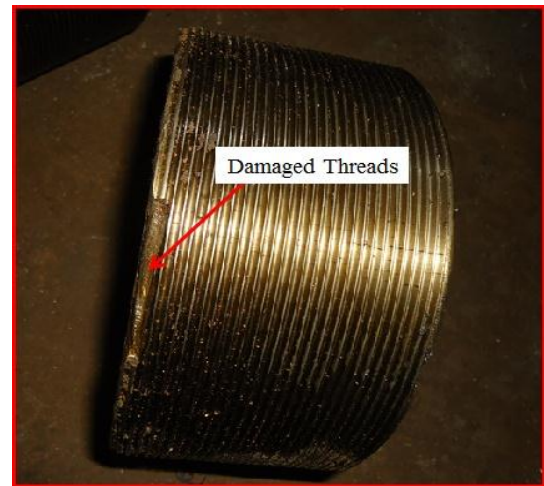
Fig. 1 Damaged threads on thread rolls
