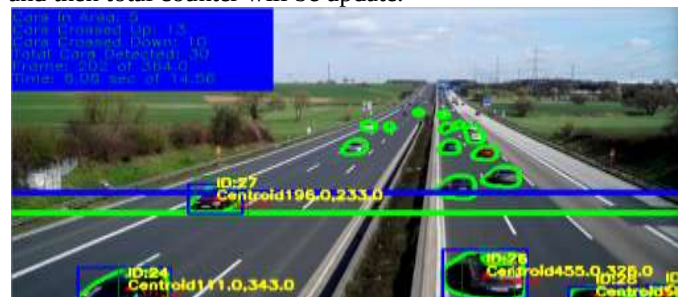
Fig.7. When the vehicle centroid crosses the imaginary line in ROI, the respective counter variables increase.
