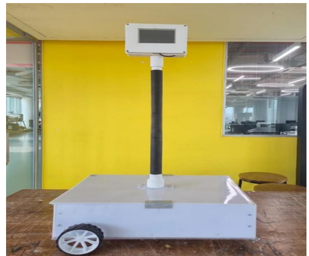
Fig. 4. Final assembled prototype of the autonomous wound-monitoring robot.
