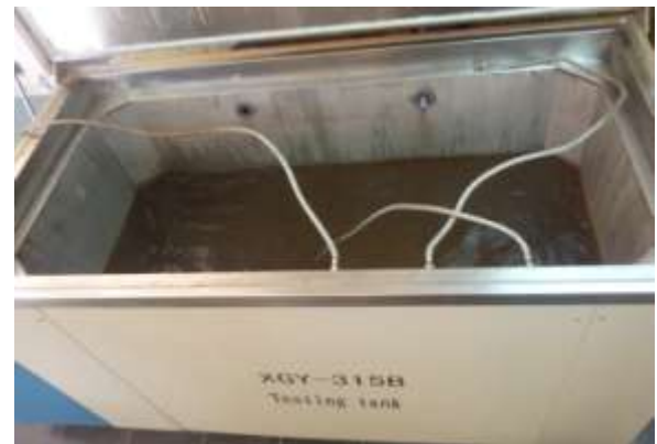
Fig: 3. Test tank for hydrostatic pressure tester
