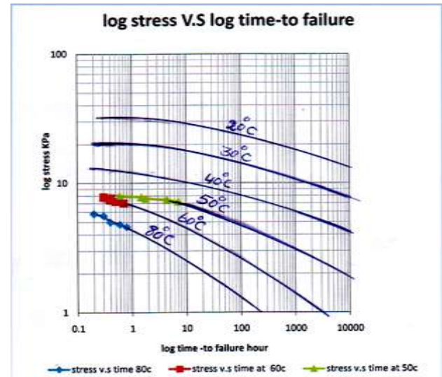
Chart: 2. Stress curve versus time to predict at temperatures (20°C, 25°C, 30°C and 40°C) of high polyethylene pipes.
