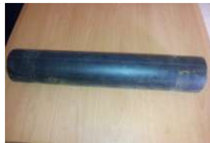
Fig:1 sample of test High density polyethylene pipe.
