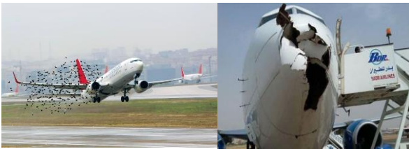
Fig 1. An example of Bird Strike and damage to the plane
