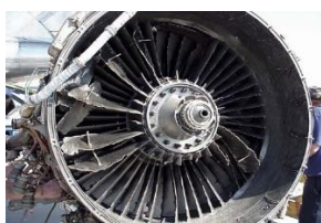
Fig 3. Jet Engine after Bird Strike [21]
