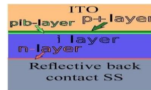
Fig.1- Silicon solar cell with flat surface:
