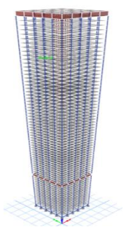
Fig. 7. Model with outriggers at H (top) and H/4
