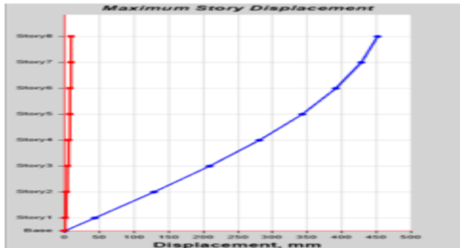
Fig 4.1 Total Displacement in EQx Direction for Clay for X bracing
