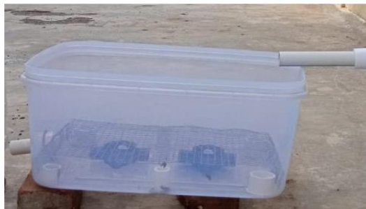
Fig No. 3. under drainage system
