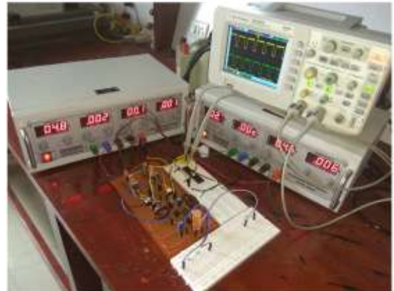
Fig. 13: Experimental setup of Dual Output DC-DC Converter
