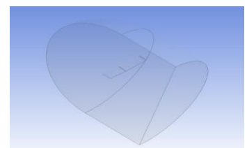
Fig.14:WingGeometry with enclose
