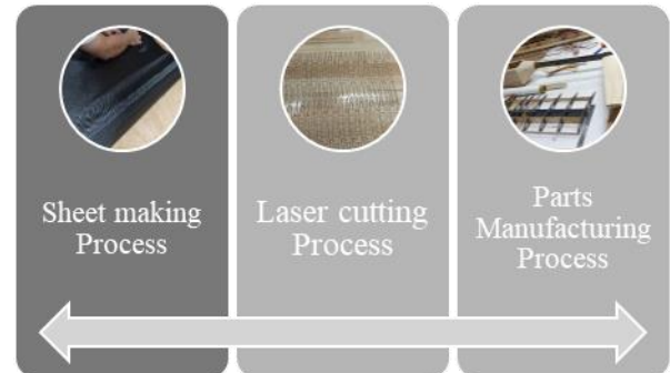
Fig.22: The flow of UAV Manufacturing Process
