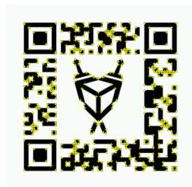
Fig. 5. Feature point detection using Vuforia Engine.
