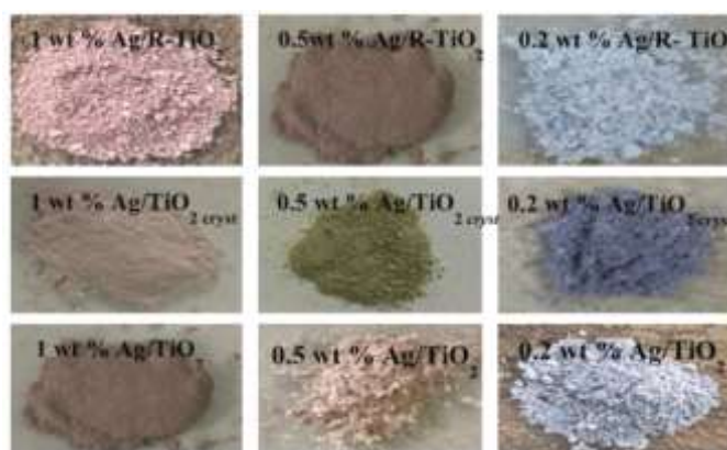
Fig. 2. Colors displayed by different catalysts upon metal loading.
