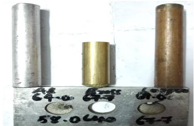
Figure 4. Aluminium as specimen and copper, brass, aluminium as electrodes
