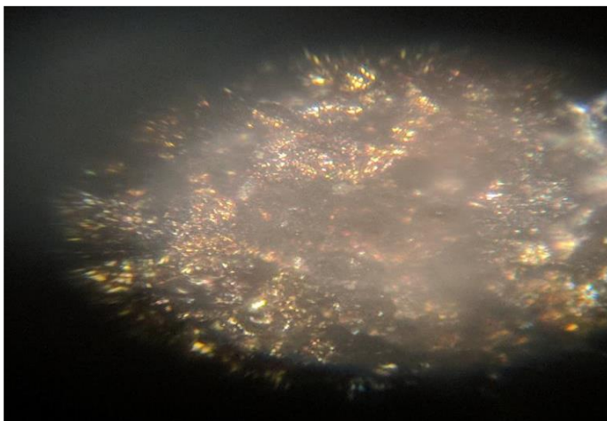
Fig 17. Brass specimen machined with Aluminium Electrode
