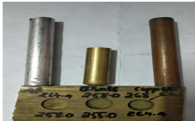
Fig 2. Brass as specimen and copper, brass, aluminium as electrodes
