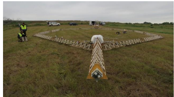
Figure 3 Technicians prepare the SkyTEM rig for aerial mapping.
