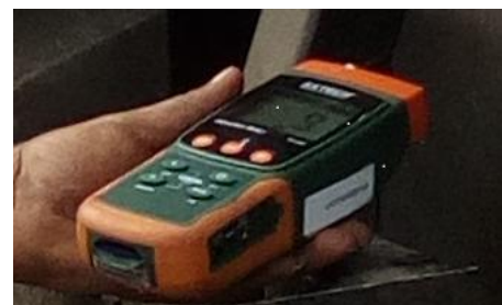
Image 1 vibration meter model SDL800
