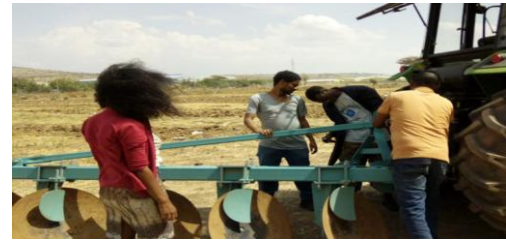
Image 3 implement attachment on chery100 hp tractor
