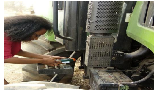
Image 4 the vibration meter magnet tip attachment to transfer case
