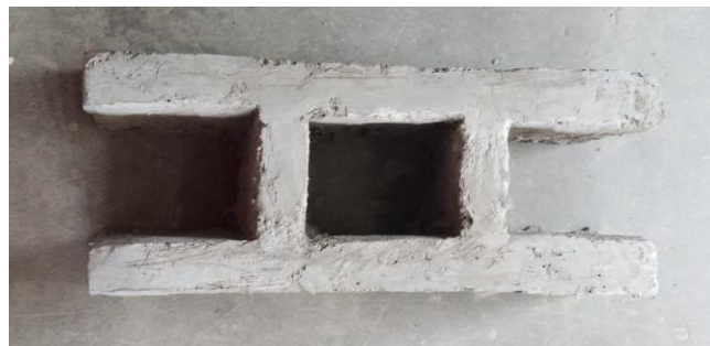
Figure 4: Cross section of paper Crete panel
