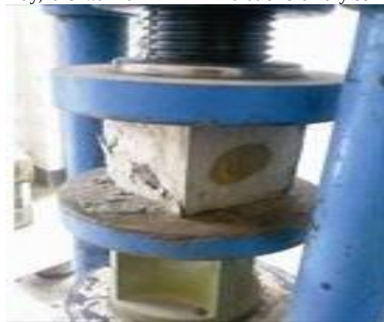
Figure 5: Compression test on concrete cube
