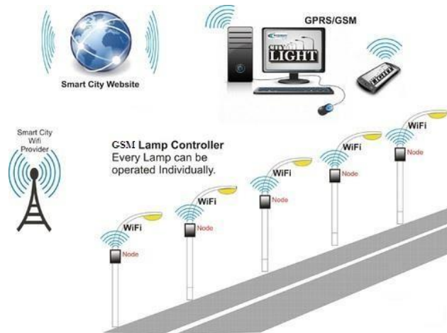
Fig 1. Street light controller with wireless technology
