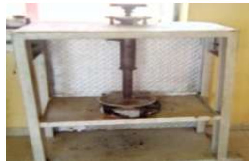
Figure 3: screw press used in briquettes compaction.
