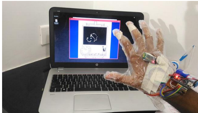
Fig. 5 Hand Gesture Controlled Laptop in action
