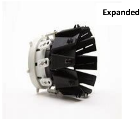
Figure 3 [A] Nozzle design with a variable area (3D printed nozzle). [23]
