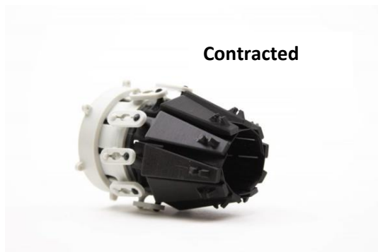
Figure 3 [B] Nozzle design with a variable area (3D printed nozzle). [24]
