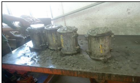
Fig .4.Casting Of Cylinder
