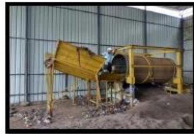
Figure 5: Screening machine used to turn the waste
