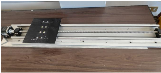
Fig. (1): A single axis ball screw feed drive system.
