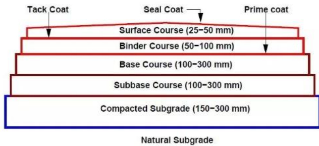
Fig. 1 Typical Cross Section of Flexible Pavement
