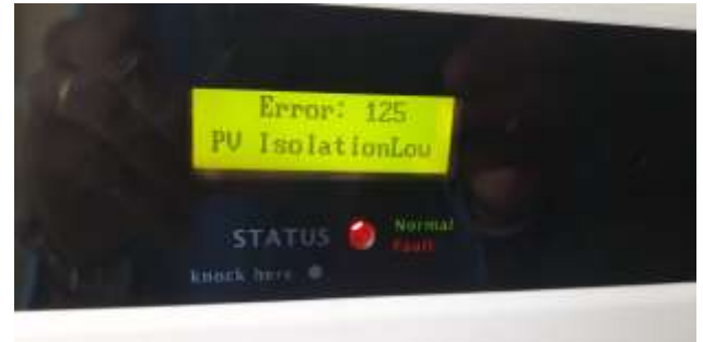
Figure 7: Error: 125 display on the inverter screen
