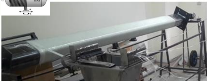
Fig. 1. Circumferential pattern of winding [90°]
