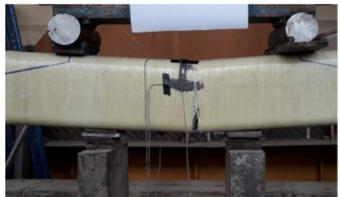
Fig. 5. Tension Failure pattern on bottom flange
