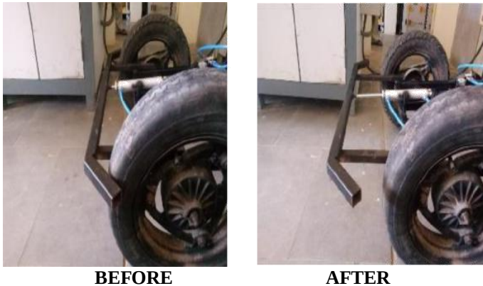
Fig.7. Bumper activation system
